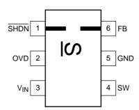
Note 1: This IC could be destroyed in some case if amounted in 180° inverse direction. Please be careful about IC direction in mounting.
